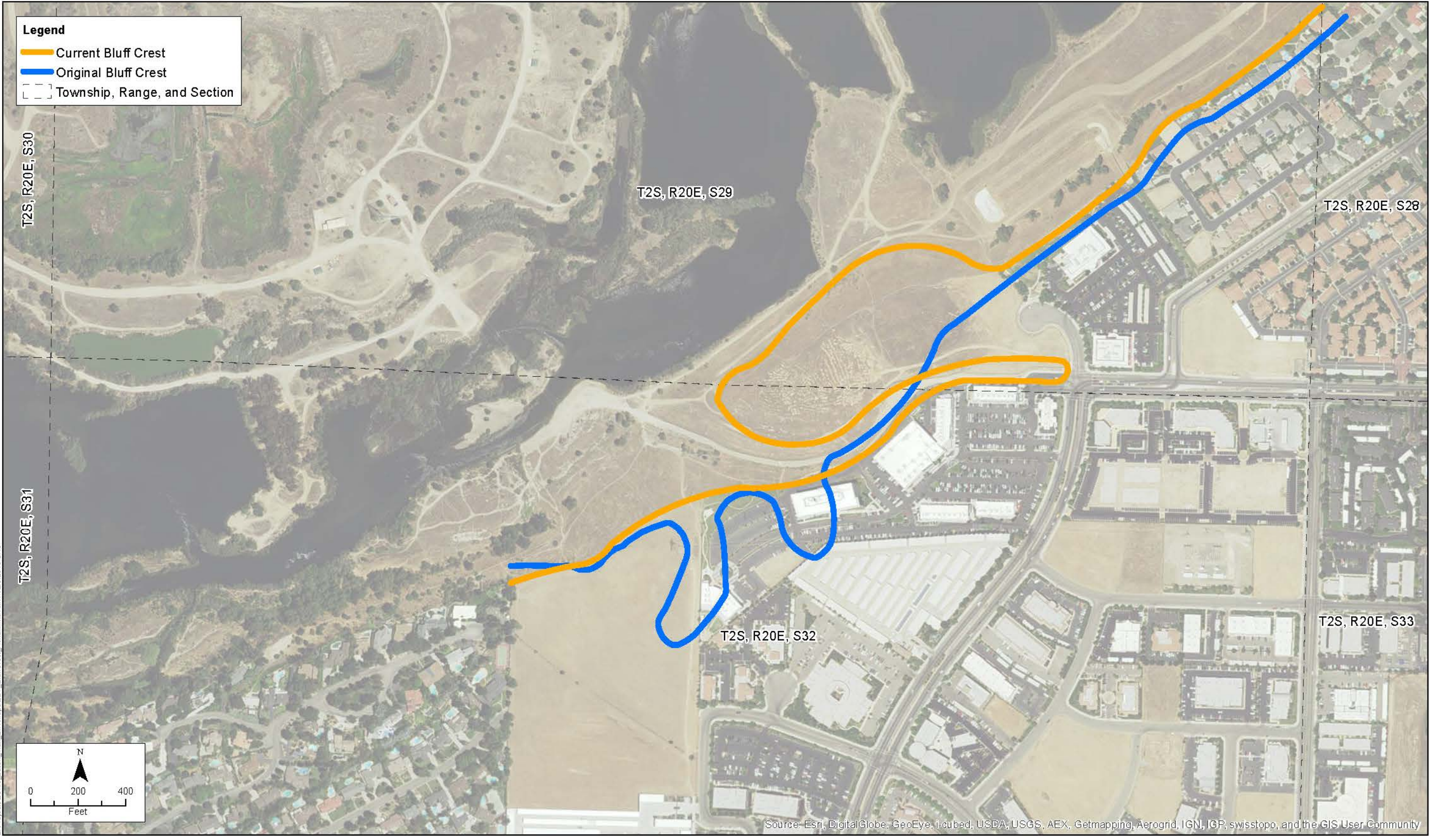
Figure 5-12 Conceptual Illustrations Comparing Current Bluff Crest with Original Bluff Crest
